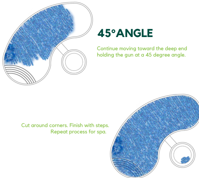
Figure 2: Continue working in 36-42” wide passes down the length of the pool to completely flock coat the floor.
